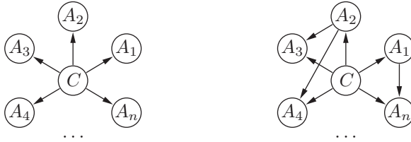
Figure 6.1 A naive Bayes classifier is a Bayesian network with a star-like structure. Additional edges can mitigate the independence assumptions.
