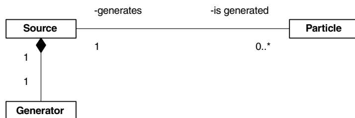
Figure 13.2. Relations among the Source , Particle and Generator classes
